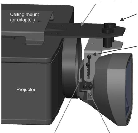
Screws, spacers and thumb knobs to place Paladin height into projector beam which typically comes out of the lower part of the projector lens.
