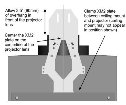
**projector for maximum security**. Alternatively, secure the XM2 plate to a shelf underneath the projector leaving the same extension in front of the projector lens.
